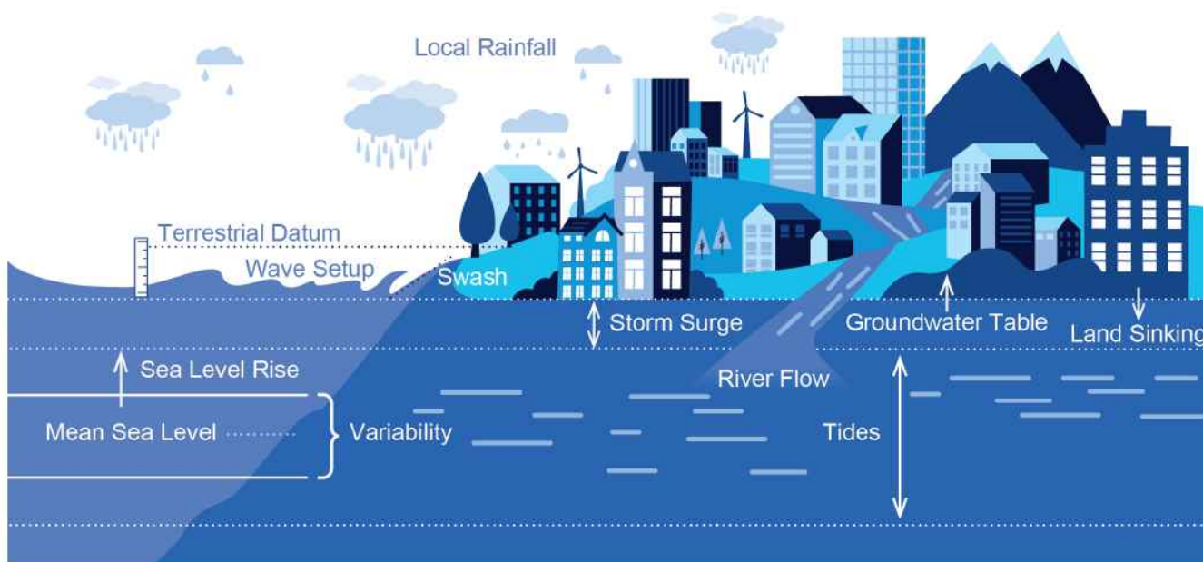
Figure 1.1: Schematic (not to scale) showing physical factors affecting coastal flood exposure. Due to the clear and strong relative sea level rise signal (i.e., combination of sea level rise and sinking lands), the probability of flooding and impacts are increasing along most U.S. coastlines.
